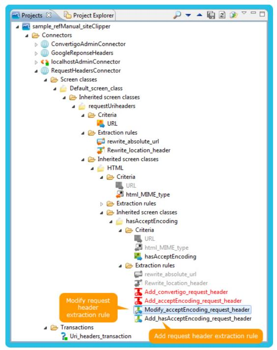
Figure 2 - 625: Modify request header extraction rule - Objects in Projects view
