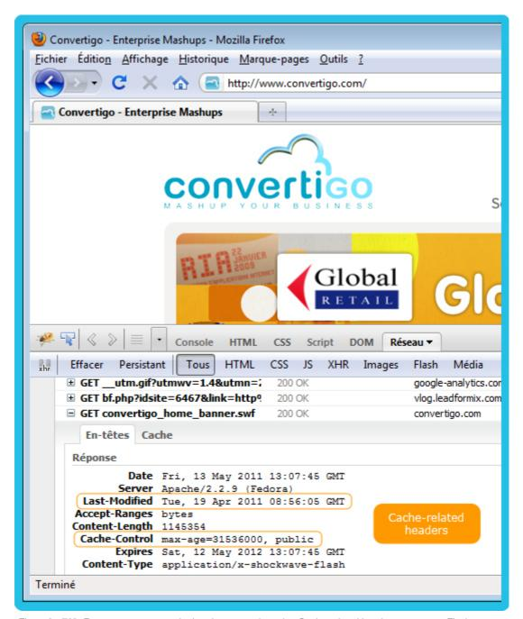
Figure 2 - 702: Remove response cache headers extraction rule - Cache-related headers present on Flash resource HTTP response
