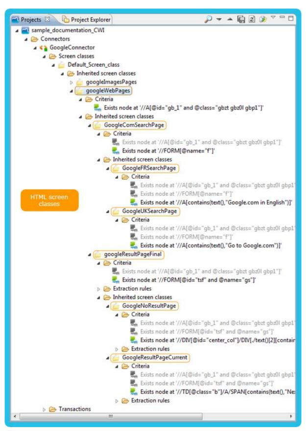
Figure 2 - 203: HTML Screen class - Project's screen classes and respective criteria
