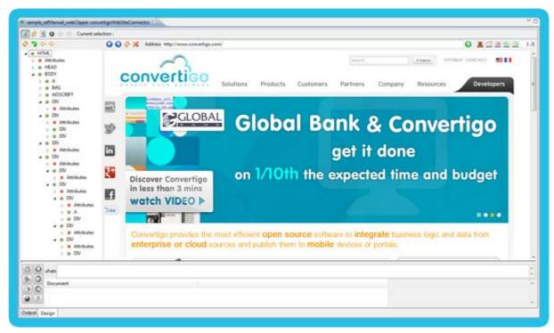
Figure 2 - 199: HTML connector - Example 2 - Connector editor with Web browser, DOM tree and XPath evaluator
