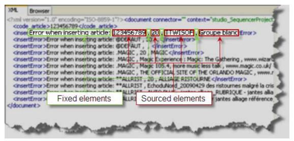
Figure 2 - 160: Fixed and sources elements of concatenated error messages
